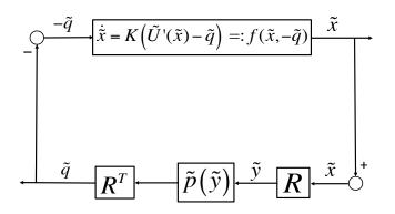
**Figure 4.6:** The primal algorithm (4.15) is modeled as a feedback connection of a dynamical system and a memoryless system.
