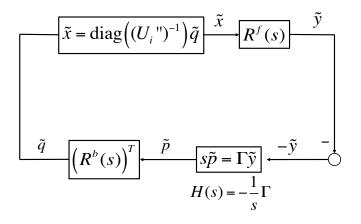
Figure 6.12: Delayed linear system representing the dual algorithm (6.25).
