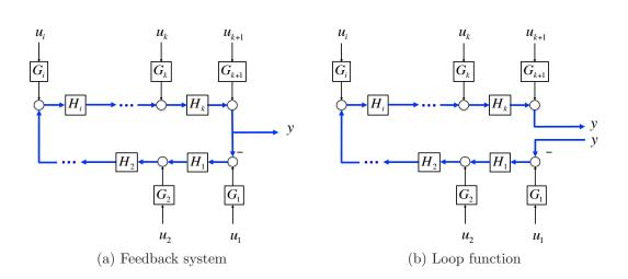
Figure 6.3: Loop function of a feedback system.
