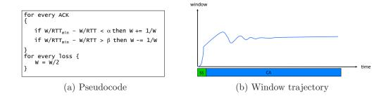
Figure 1.4: Congestion avoidance behavior of TCP Vegas.
