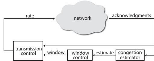
Fig. 1. System view in window-based congestion control.
