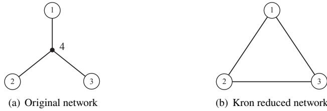
Figure 4.10 Kron reduction: N_{\text{red}} := \{1, 2, 3\} with internal bus 4. While the original network is a tree, the Kron reduced network is fully connected.
