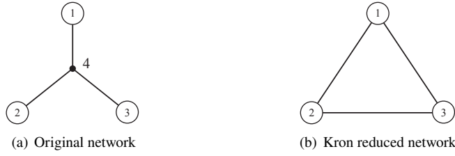
Figure 4.10 Kron reduction: N_{\text{red}} := \{1, 2, 3\} with internal bus 4. While the original network is a tree, the Kron reduced network is fully connected.
