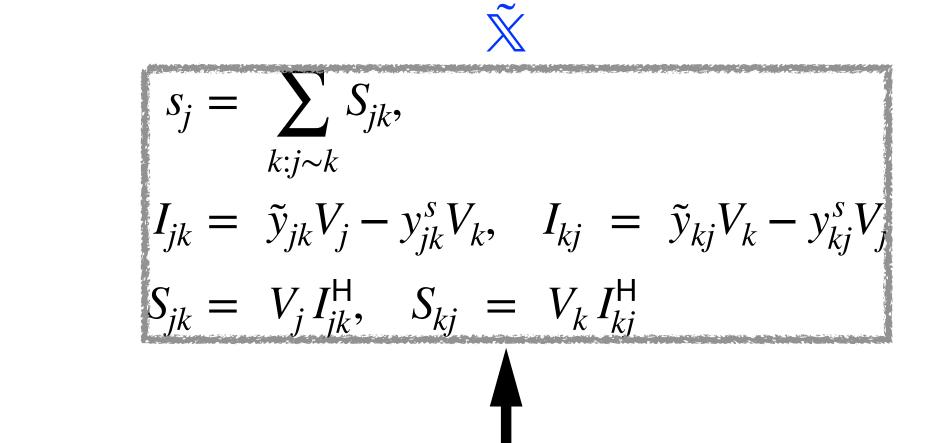
$$s_{j} = \sum_{k:j \sim k} (y_{jk}^{s})^{H} (|V_{j}|^{2} - V_{j}V_{k}^{H}) + (y_{jj}^{m})^{H} |V_{j}|^{2}$$
