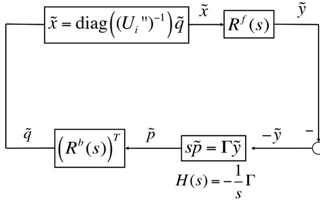
**Figure 6.12:** Delayed linear system representing the dual algorithm (6.25).
