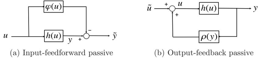
**Figure 4.2:** (a) Input-feedforward passive system  $u^T \tilde{y} \geq 0$ . (b) Output-feedback passive system  $\tilde{u}^T y \geq 0$ .
