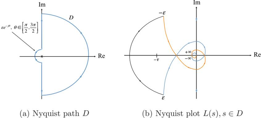
**Figure 6.9:** (a) Nyquist path  $D$  that indents left at the origin. The indentation is the path  $(\epsilon e^{-j\theta}, \theta \in [\pi/2, 3\pi/2])$  for an arbitrarily small  $\epsilon > 0$ . (b) The corresponding Nyquist plot  $(L(s) = \frac{1}{s} e^{-\tau s}, s \in D)$ . The plot  $L(s)$  on the indentation  $s = (\epsilon e^{-j\theta}, \theta \in [\pi/2, 3\pi/2])$  is the black curve with a counterclockwise orientation.
