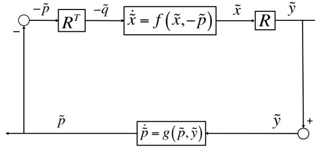
**Figure 4.7:** The primal-dual algorithm (4.19) is modeled as a feedback connection of two time-invariant dynamical systems.
