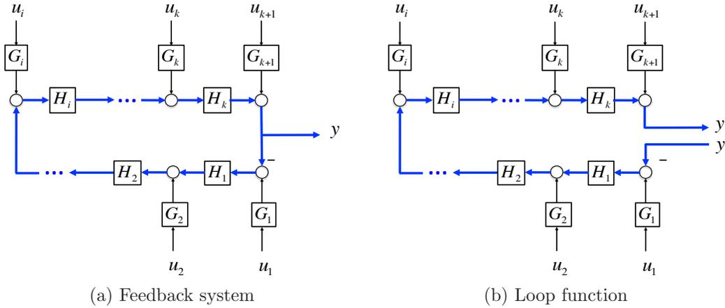
Figure 6.3: Loop function of a feedback system.
