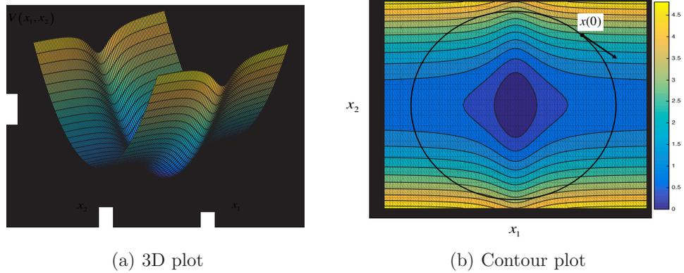
**Figure 3.5:** Plots of  $V(x) = x_1^2/(1+x_1^2) + x_2^2$ . Starting from an  $x(0)$  such that  $V(x(0)) > 1$ , the trajectory  $x(t)$  may not stay in any bounded set even if  $\dot{V} < 0$ .
