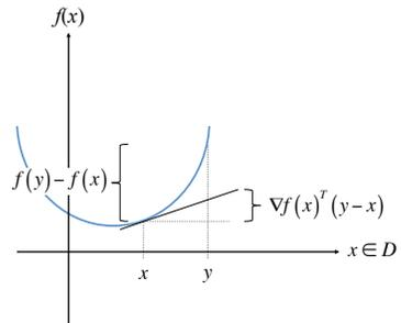
**Figure 2.2:** Definition of a convex function: The straight line connection  $f(x)$  and  $f(y)$  lies above  $f$  between  $x$  and  $y$ . The linear approximation of a differentiable convex function  $f$  lies below  $f$ .
