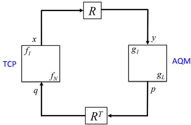
**Figure 1.7:** The basic model: a multi-source multi-link network.
