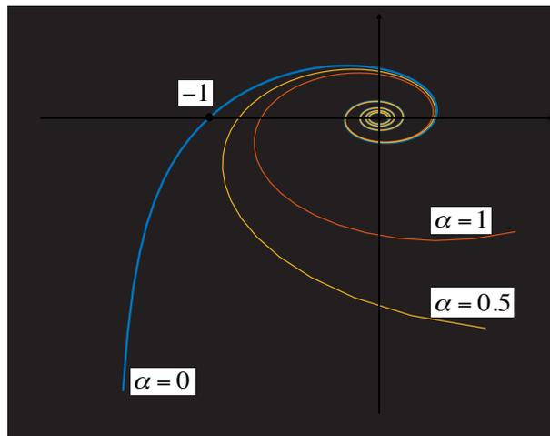
**Figure 6.11:** The Nyquist plots  $\left\{ \frac{\pi}{2} \frac{e^{-j\omega}}{j\omega + \alpha_i}, \omega \in [0, +\infty] \right\}$  for  $\alpha_i = 0, 0.5, 1$  in the complex plane. They cross the real axis to the right of  $-1$  as long as  $\alpha_i > 0$ . When  $\alpha = 0$ , see Figure 6.9 in Example 6.20 for the complete Nyquist plot.
