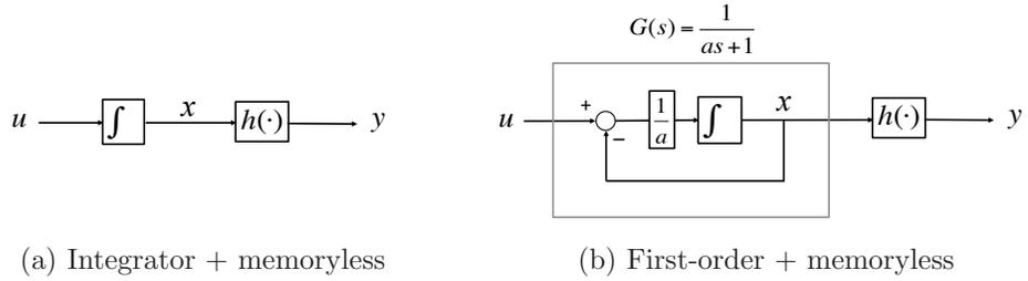
**Figure 4.3:** (a) Integrator in cascade with a memoryless passive system is passive with the storage function  $V(x) := \int_0^x h(\sigma)d\sigma$ . (b) First-order system in cascade with a memoryless passive system is passive with the storage function  $V(x) := \int_0^x ah(\sigma)d\sigma$ .
