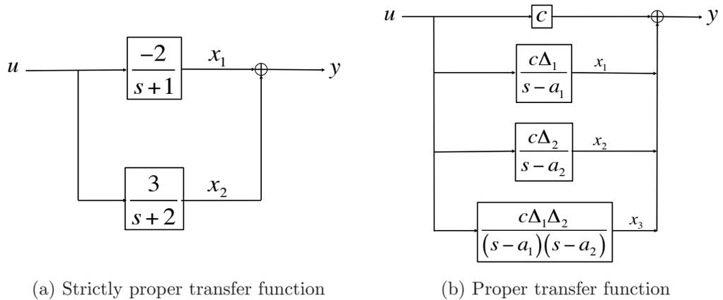
**Figure 6.2:** Realization of the transfer functions in Example 6.3. (a) Strictly proper transfer function  $H(s) = \frac{s-1}{(s+1)(s+2)}$ . (b) Proper transfer function  $H(s) = \frac{c(s-b_1)(s-b_2)}{(s-a_1)(s-a_2)}$ .
