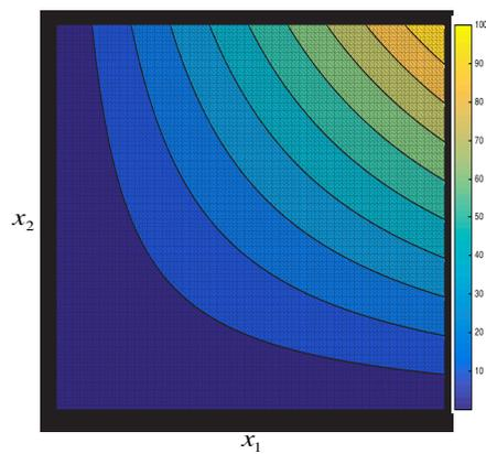
**Figure 2.3:** Contour plot of  $f(x) = x_1 x_2$  which is neither convex nor concave over  $D := \{(x_1, x_2) \mid x_1 > 0, x_2 > 0\}$ .
