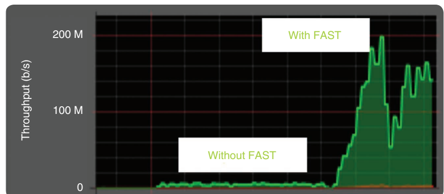
FIGURE 3 When the Sprint network experienced heavy packet losses in June 2007, FAST TCP increased throughput between San Francisco and New York by 120 times.
